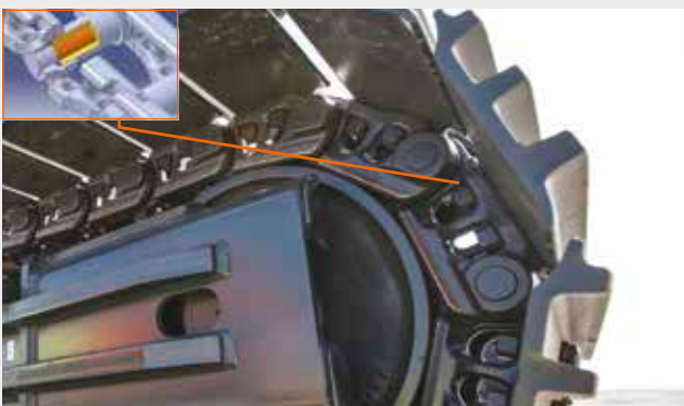
Complete Lubrication for the centred rollers
